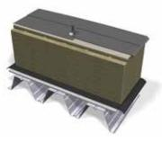
Steel trapezoid roofs are widely used for various types of building. These roofs usually consist of steel beams, steel trapezoid profile, vapor barrier, thermal insulation and roof membrane. Since each component in this structure has very different fire behavior, it is best to test the whole system to see how it behaves in a fire.
