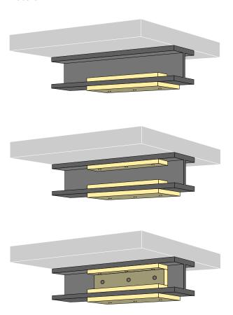
c. Finally, fit the slabs covering the edge of the flanges. Use PAROC Welding pins, maximum c/c 367 mm, and maximum 50 mm from the slab joints.
