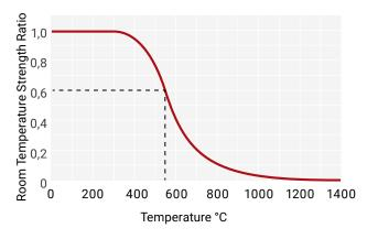
Fires in buildings frequently exceed 1000 degrees Centigrade within a relatively short period of time (30–60 minutes), yet heavily loaded steel loses its design safety margin, approx. 40%, at temperatures around 550°C, regardless of the grade. As the temperature rises further, the loss of strength is rapid and significant.
