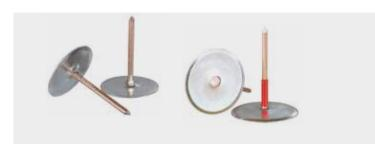
d. The protection slabs on the sides are fastened with welding pins on the upper and lower flange. Pins should be fitted at a maximum separation of 367 mm and maximum 50 mm from the slab joint. The protection slabs have to be fixed to the supporting boards in the web by PAROC Fire Springs. The length of the PAROC Fire Spring shall be at least twice the insulation thickness. The number of springs depends on the profile height.
