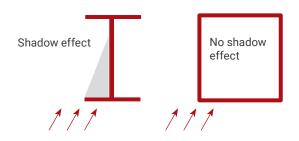
Whilst the section factor can be calculated, it is more usual to refer to the various steel manufacturers' profile information, where this value is given.
