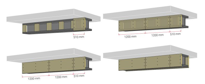
b. Fit the slabs on the side of the beam or column, by fastening them to the supports with minimum 3 fire springs. The length of the fire spring should be at least insulation thickness + 60 mm (support board thickness). The height of the slabs should be the profile height + 1 x insulation thickness.
