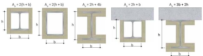
$A_n = inner contour of encasement (m) x 1 m)$
