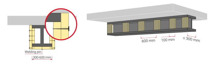
a. Fit the supports between the flanges, they have to be positioned at slab joints and at the center of each slab, max 600 mm separation. Thickness of supporting boards should be 60 mm. Make sure to cut the supporting boards 2–3 mm longer than the distance between the flanges to obtain a tight fit.
