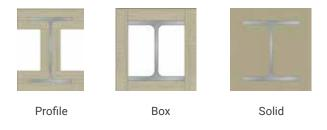
Sprayed materials are normally applied to follow the profile of the section. Special insulating concretes can be used to form solid protection.
