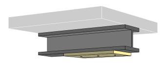
Fit the insulation inside the web of the beam, using the same distances between PAROC Welding pins described above.
